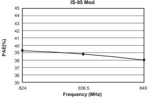
RMPA0967 Cellular 3x3mm<sup>2</sup> PAM Vcc=3.4 V, Vref=2.85V, Vmode=0V, Pout=28 dBm, IS-95 Mod
